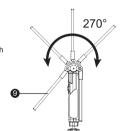
Turn the part "2" ON/OFF adjustment wheels clockwise, can turn the light on and adjust it from low brightness to high one; Turn it counterclockwise, can be from high brightness to low one and till closed off
